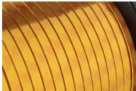
flat aluminium wire insulated with 2 layers SynTherm® H, in opposite directions, 25 % overlap
